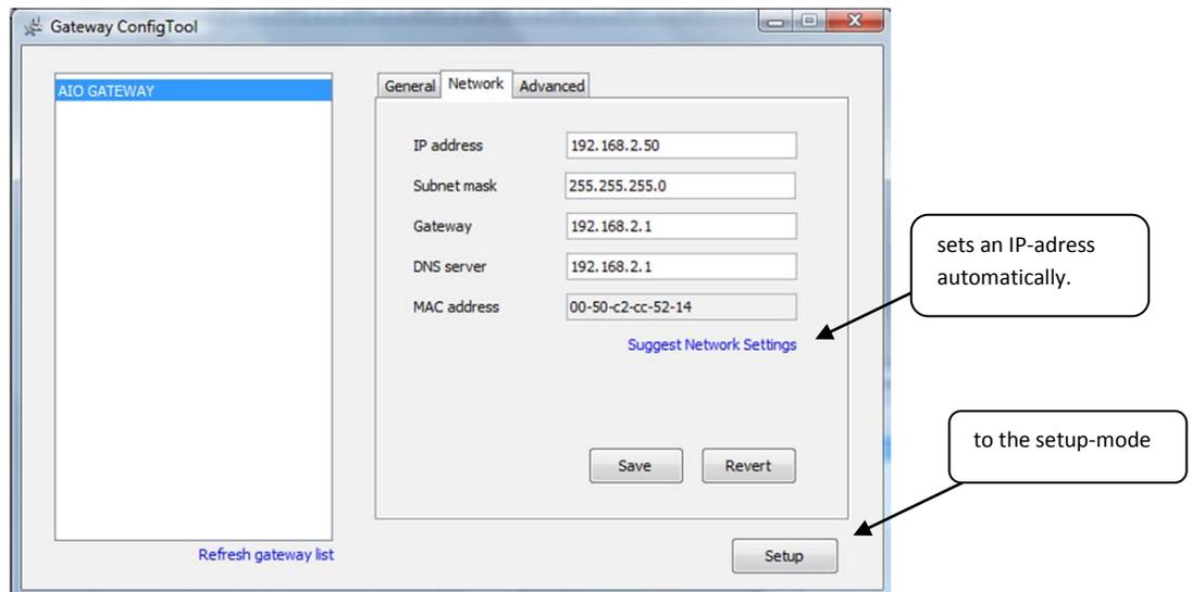
Now adapt the IP-Settings to your local network (Tab "Network"). Select the „Network“ Tab and click the Setup-Button. Here a password is required. The original password in the factory settings is: **„admin“**. Now you enter the setup-mode and are able to change all settings (passwords, names, etc)
